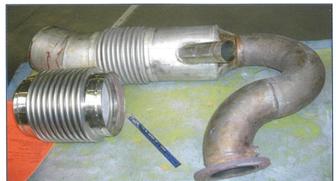
3 pin 'hinged' expansion joint system to absorb large movements of the piping, without transmitting pressure thrust loads on adjacent pipework. This solution is ideal for suspended piping, where it can be difficult to position sufficiently strong fixed points.
