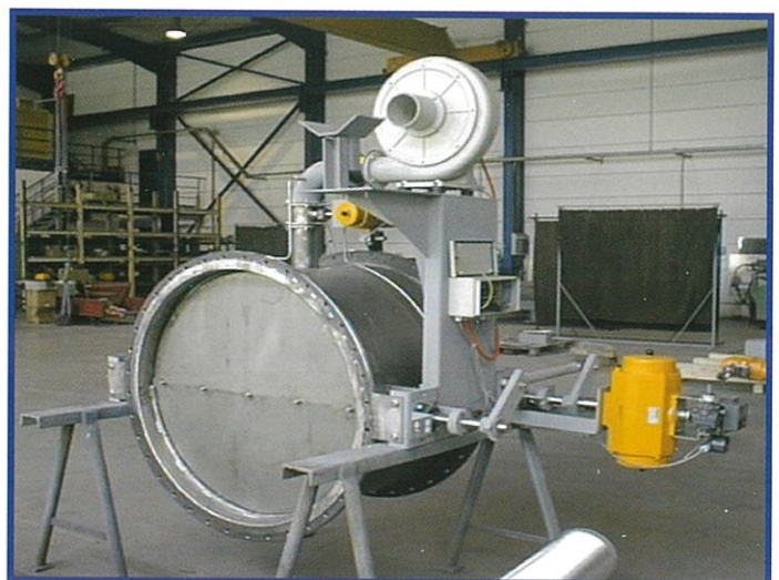
flue gas valves
