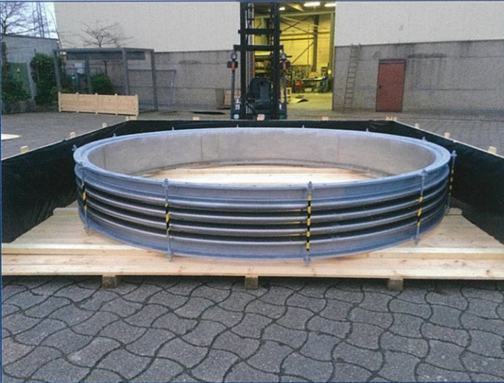
Stainless steel expansion joint DN4000 for a cement factory, comprising an inner sleeve and insulation in the convolutions (to prevent ingress and settlement of dirt and dust particles).
